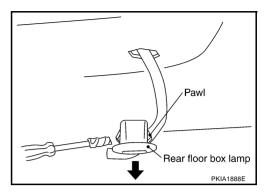
2. Turn bulb socket counterclockwise to release lock and remove it.
