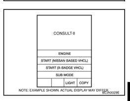
Touch "BCM" on "SELECT SYSTEM" screen. If "BCM" is not displayed, print "SELECT SYSTEM" screen, then refer to GI-39, "CONSULT-II Data Link Connector (DLC) Circuit"
