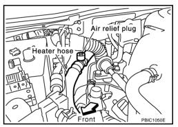
3. Fill radiator with water until water spills from the air relief hole, then close air relief plug. Fill radiator and reservoir tank with water and reinstall radiator cap.
