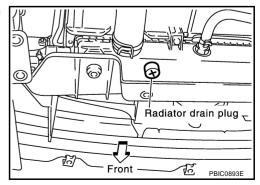
When drain all of engine coolant in the system, open water drain plugs on engine cylinder block. Refer to <a href="EM-139">EM-139</a>, "DISASSEMBLY"</a>.
