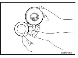
2. Install side gear and thrust washer into differential case B. CAUTION:
