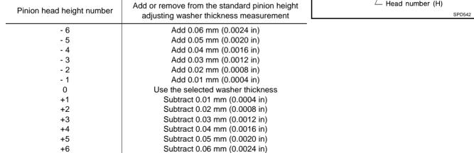
12. Select the correct pinion height adjusting washer. Refer to RFD-57, "Pinion Height Adjusting Washer".
