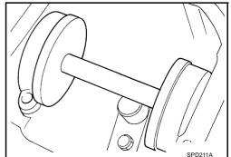
9 Select the correct standard pinion height adjusting washer thickness. Select by using a standard gauge of 3 mm (0.12 in) and your J-34309-101 feeler gauge. Measure the distance between the J-34309-11 pinion height adapter including the standard gauge and the arbor.
