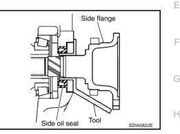
c. Put a suitable drift on the center of side flange, then drive it until sound changes.
