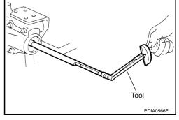
7. Place the J-34309-11 "R200A" pinion height adapter onto the gauge plate and tighten it by hand. **CAUTION:**
