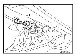
5. Remove front oil seal using the puller.
