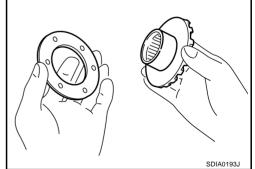
2. Install side gears and thrust washers into differential case. CAUTION:
