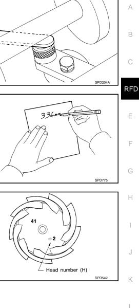
11. Correct the pinion height washer size by referring to the "pinion head number".
