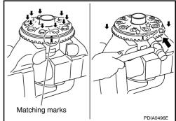
13. Remove lock pin of pinion mate shaft with a punch from drive gear side.
