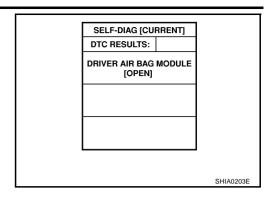
If no malfunction is detected on "SELF-DIAG [CURRENT]" even though malfunction is detected in "SRS Operation Check", check the battery voltage. If the battery voltage is less than 9 V, charge or replace the battery. <u>SRS-27</u>, "<u>DIAGNOSTIC PROCEDURE 3</u>". If the battery voltage is OK, go to <u>SRS-29</u>, "<u>DIAGNOSTIC PROCEDURE 4 (CONTINUED FROM DIAGNOSTIC PROCEDURE 2)</u>" diagnose the following cases:
