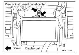
3. Remove screws (4), and remove bracket.
