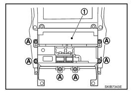
3. Remove screws (8), and remove bracket.
