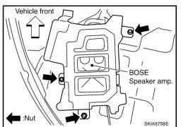
4. Remove bolts (4), and remove bracket.
