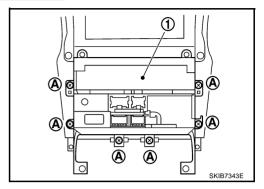
4. Remove screws (8), and remove bracket.
