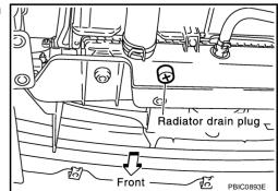
When drain all of engine coolant in the system, open water drain plugs on engine cylinder block. Refer to <u>EM-138, "DISASSEMBLY"</u>.
