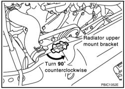
b. Lift A/C condenser up and remove radiator after disengaging the fitting as front-bottom surface.
