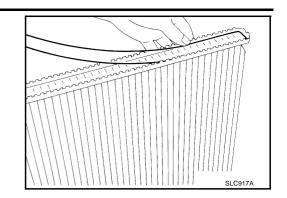
3. Caulk tank in numerical order as shown in the figure with radiator plate pliers A (SST).
