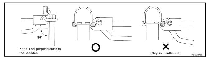
• Use pliers in the locations where radiator plate pliers A [SST: KV99103510 ( — )] cannot be used.
