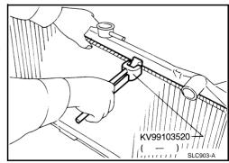
• Grip the crimped edge and bend it upwards so that radiator plate pliers B [SST: KV99103520( — )] slips off. А **CAUTION:** ø Do not bend excessively. СО С t SLC893 D • In areas where radiator plate pliers B [SST: KV99103520( )] cannot be used, use screwdriver to bend the edge up. **CAUTION:** Е Be careful not to damage tank. F G SLC930 2. Remove sealing rubber. Н 3. Make sure the edge stands straight up. I J
