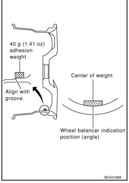
c. If calculated balance weight value exceeds 50 g (1.76 oz), install two balance weight sheets in line with each other (as shown in the figure).
