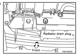
When drain all of engine coolant in the system, open water drain plugs on engine cylinder block. Refer to  $\underline{\sf EM-138}$ , "DISASSEMBLY".
