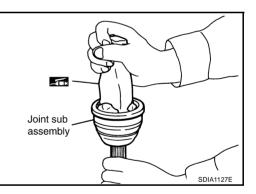
Wind serrated part of shaft with tape. Install boot band and boot to shaft. Be careful not to damage boot.
