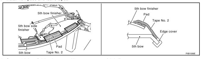
10. Secure 5th bow finisher harness with new nonwoven fabric if necessary.
