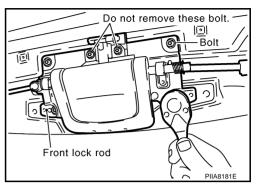
3. Remove bolts, and then remove front lock striker, LH, center, and RH.
