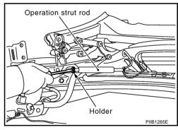
Temporarily fix 5th bow operating strut rods on 5th bow finisher after removal.
