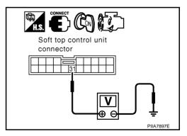
Soft top control unit connector connector
