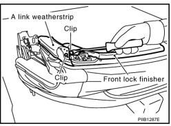
9. Pull up front lock lever, and then disengage clips to remove front lock finisher.
