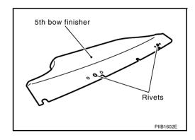
Replace retainers under 5th bow finisher with a new part.
