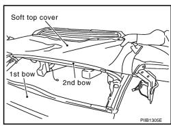
35. Pull up 2nd bow retainer by using a screwdriver, and then remove soft top cover from 2nd bow.
