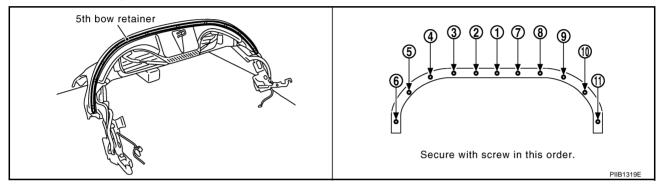
23. Shave rivets head of soft top cover 5th bow by using a drill. [Drill bit diameter: 5.5 mm (0.22 in)]
