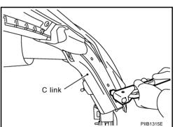
19. Align screw hole on soft top cover and the bottom of C link, and then tighten with screw.
