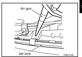
2. Remove the remains drawn to both ends by the air blow from the gap.
