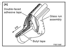
Water may be entering through connection between front pillar and front edge of soft top. Cause: There may be a gap between glass run assembly and weather strip of soft top.
