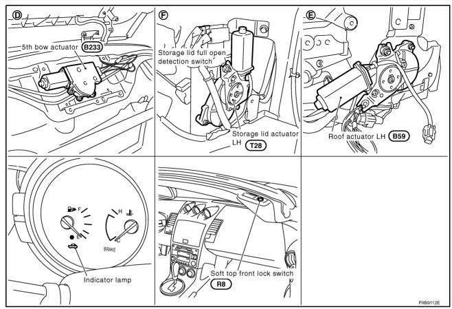
Following Parts Are Built Into 5th Bow Auto Closure Assembly.
