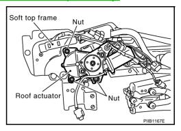
3. Disconnect soft top actuator harness connector.
