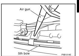
• Remove the remains drawn to both ends by the air blow from the gap.
