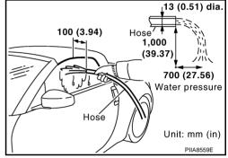
4. Visually check for water leakage.
