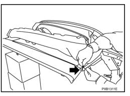
8. Tighten soft top cover wire rear bracket to C link with screw. (Face tension wire outside.)
