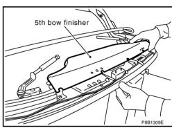
4. Remove rivets head of 5th bow finisher retainer.
