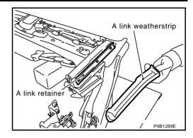
11. Peel a link sealing out.
