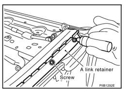
14. Remove screws, and then remove A link retainer.
