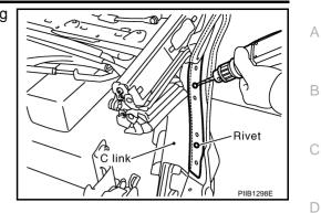
25. Cut EPT seal and remove screws on the bottom of C link. **NOTE:**
