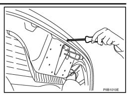
8. Drilling rivets attaching the soft top cover to 5th bow, then pull up the soft top cover bottom edge.
