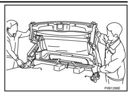
6. Protect the limit switch contact around the rotation axis of the 5th bow on the left side of soft top with tape.
