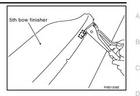
Remove remains of soft top cover mounting rivet from 5th bow and C link.
