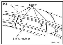
Insert approximately 0.5 mm (0.02 in) washer into the back of the subsiding weather strip retainer, if the step is not eliminated after adjustment.
