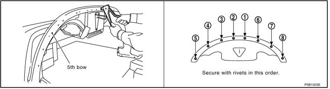
18. Secure soft top cover to C link with rivet.
