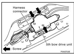
18. Remove 5th bow drive unit and rails together from 5th bow by removing screws.
