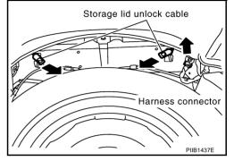
Disconnect roof actuator harness connector right and left side (disconnect top of roof actuator harness connector right and left side).
