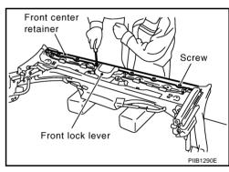
13. Put matching marks to installation position of A link retainer.
