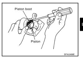
3. Apply a brake fluid to the piston, insert into the cylinder body by hand and firmly attach the piston boot piston-side lip into the piston groove.
