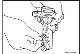
4. Insert the plate and guide into the cylinder body.
