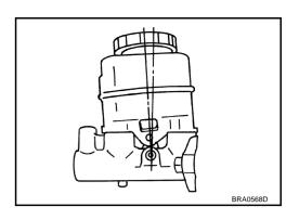
8. Using a pin punch [commercial service tool: diameter Approx. 4 mm (0.16 in)], attach the reservoir tank mounting pin so that the attachment side and the opposite side are identical.
