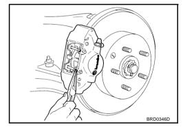
3. Remove the pad pin while holding down the cross spring, then remove the cross spring from the caliper.
