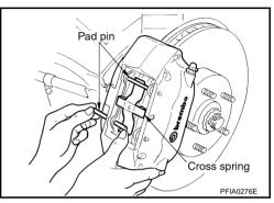
Removal and Installation of Brake Caliper Assembly (Other than Brembo Calipers)
