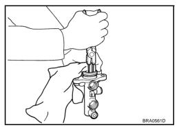
Tap flange using a soft block such as wood, and carefully pull the secondary piston assembly straight out to prevent cylinder inner wall from being damaged.
