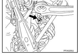
3. Refill brake fluid and bleed air. Refer to BR-11, "Bleeding Brake System" .
