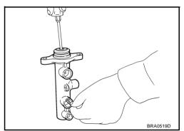
4. Holding down the piston with the stopper cap, push the stopper cap tabs so they are firmly into the cylinder grooves, then attach the stopper cap.
