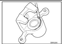
4. Place a wooden block as shown in the figure, and blow air from union bolt mounting hole to remove pistons and piston boots.
