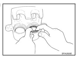
2. Apply rubber grease to piston boots. Cover the piston end with piston boot, and install cylinder-side lip on piston boot properly into groove on cylinder body.
