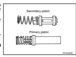
• Pay attention to the orientation of the piston cup, and insert straight to prevent the cup from being caught by cylinder inner wall.
