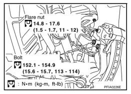
Attach the brake tube to the caliper assembly and partially tighten the flare nut.
