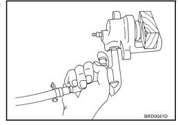
5. Using a flat-bladed screwdriver, remove piston seals from cylinder body.
