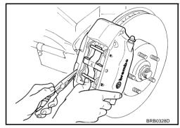
4. Using pliers, remove the pad from the caliper.
