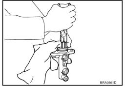
6. Place the side of the cylinder body with chamfering around the pin insertion hole up, and secure the cylinder body flange section with a vise.
