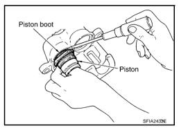
3. Apply brake fluid to piston, and press piston into cylinder body by hand to assemble piston-side lip on piston boot properly into a groove on piston.
