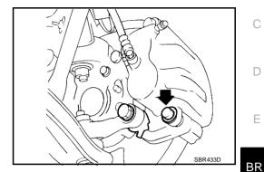
3. Hang cylinder body with a wire, and remove pads, shims and pad retainers from torque member.
