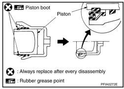
4. Fix piston boot with retaining ring.
