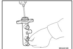
Tap flange using a soft block such as wood, and carefully pull the secondary piston assembly straight out to prevent cylinder inner wall from being damaged.
