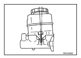
8. Tilt the reservoir tank so that the mounting pin can be inserted as shown in the figure, and insert the mounting pin. When the mounting pin has passed the master cylinder pinhole, return the reservoir tank to a level position. Attach the mounting pin to the opposite mounting pin hole of the reservoir tank so that it is the same as the insertion side.
