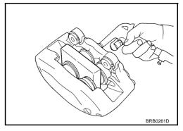
3. Using a flat-bladed screwdriver, remove the piston seal.
