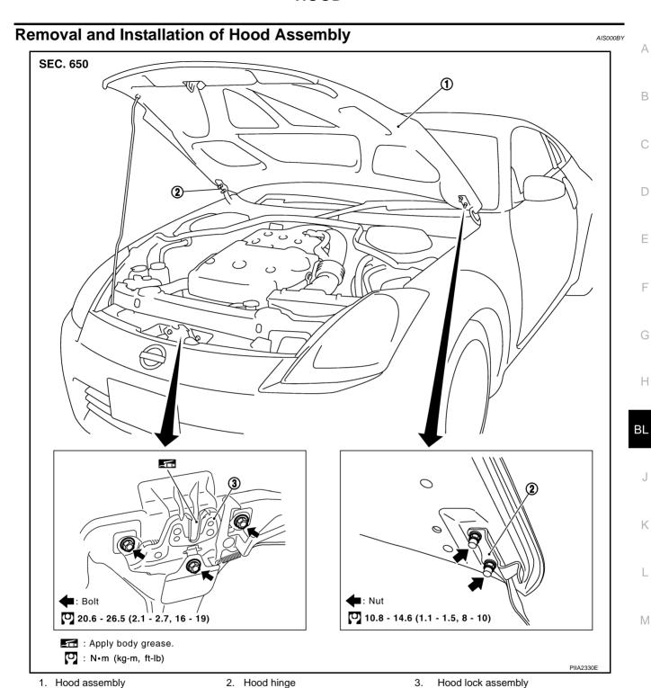
1. Remove the hinge mounting nuts on the hood to remove the hood assembly.
