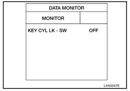
Check door key cylinder switch ("KEY CYL UN-SW") in "DATA MONITOR" mode with CONSULT-II.
