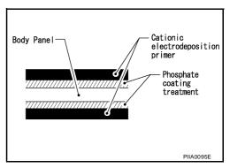
Nissan Genuine Service Parts are also treated in the same manner. Therefore, it is recommended that GENU-INE NISSAN PARTS or equivalent be used for panel replacement to maintain anti-corrosive performance built into the vehicle at the factory.
