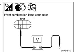
2. When tail lamp relay is operating, check voltage between front combination (side marker) lamp and ground.
