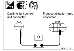
Daytime light control unit connector Front combination lamp connector
