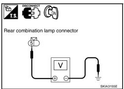
5 When tail lamp relay is operating, check voltage between license plate lamp terminal 2 and ground.
