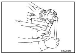
7. Tighten the drive pinion nut by very small degrees until the specified preload in achieved, when checking the preload, turn drive pinion in both directions several times.
