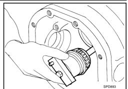
4. Assemble the front pinion bearing inner race and the J34309-2 gauge anvil. Assemble them together with the J34309-1 gauge screw in the final drive housing. Make sure that the pinion height gauge plate, J34309-16, will turn a full 360 degrees. Tighten the two sections together by hand.
