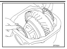
4. Align mark on bearing cap with that on gear carrier and install bearing cap on gear carrier.
