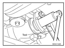
4. Using the puller, remove the companion flange.
