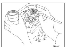
3. Hold companion flange steady by hand and rotate the drive gear in both directions.
