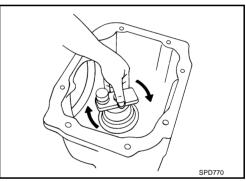
6. Measure the turning torque at the end of the J34309-2 gauge anvil using torque wrench J-25765A.
