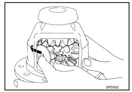
Fit pinion mate shaft to differential case so that it meets lock pin holes.
