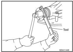
3. Using the puller remove companion flange.
