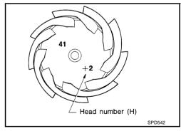
There are two numbers painted on the drive pinion gear. The first one refers to the drive pinion and drive gear as a matched set. This number should be the same as the number on the drive gear. The second number is the "pinion head height number". It refers to the ideal pinion height from standard for quietest operation. Use the following chart to determine the correct pinion height washer.
