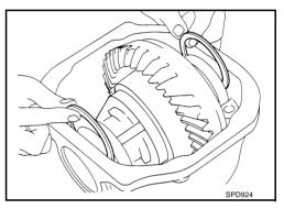
4. Install the bearing caps in their correct locations and torque the bearing cap retaining bolts.
