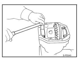
4. Lift differential case assembly out with Tool.
