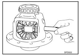
3. Adjust clearance between rear face of side gear and thrust washer by selecting side gear thrust washer. Refer to RFD-34. "AVAILABLE SIDE GEAR THRUST WASHERS".
