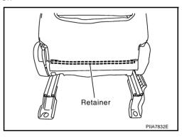
10. After removing the seatback trim and pad, remove the hog rings to separate the trim, and pad.
