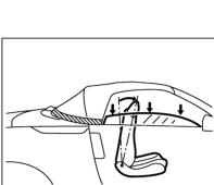
2. Soft top OPEN operation starts as soon as the passenger seatback tilt forward operation completes.
