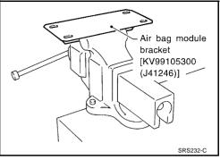
2. Match the hole in air bag module bracket (held in vise) and front passenger air bag module and fix them with one bolt [M8  $\times$  25 - 30 mm (0.98 - 1.18 in)].
