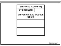
If no malfunction is detected on "SELF-DIAG [CURRENT]" even though malfunction is detected in "SRS Operation Check", check the battery voltage. If the battery voltage is less than 9V, charge or replace the battery. <u>SRS-23</u>, "<u>DIAGNOSTIC PROCEDURE 3</u>". If the battery voltage is OK, go to <u>SRS-25</u>, "<u>DIAGNOSTIC PROCEDURE 3</u>". If the battery voltage is OK, go to <u>SRS-25</u>, "<u>DIAGNOSTIC PROCEDURE 3</u>" diagnose the following cases:
