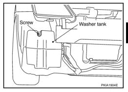
6. Remove washer tube, and remove washer tank from the vehicle.
