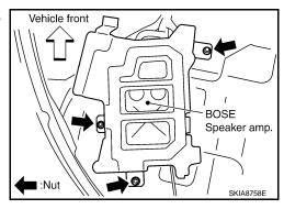
Remove bolts (4), and remove bracket.
