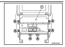
3. Remove screws (8), and remove bracket.
