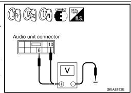
Check voltage between BOSE speaker amp., woofer amp. harness connector terminals and ground (BOSE system).
