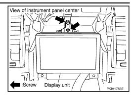
3. Remove screws (4), and remove bracket.
