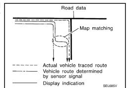
The vehicle position may not be corrected under the following circumstances and after driving for a certain time when GPS information is difficult to receive. In this case, the current-location mark on the display must be corrected manually.
