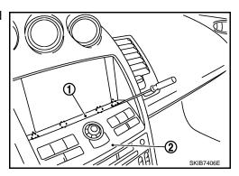
2. Remove screws (A), and remove NAVI switch (1).
