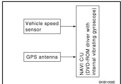
is judged and used by comparing vehicle position detection results found by the GPS with the result by mapmatching.
