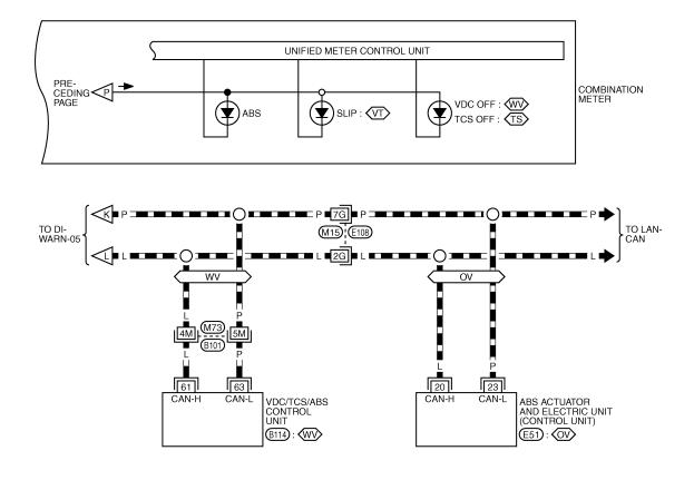
REFER TO THE FOLLOWING. (E108), (B101) -SUPER MULTIPLE JUNCTION (SMJ) (E51), (B114) -ELECTRICAL UNITS
