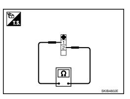
**KEY SWITCH** Check continuity between key switch terminals 1 and 2.
