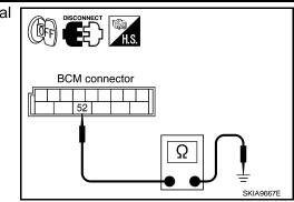
Meter Buzzer Circuit Inspection
