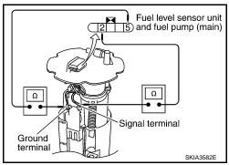
Fuel Level Sensor Unit (Sub) Check the resistance between terminals 1 and 2.
