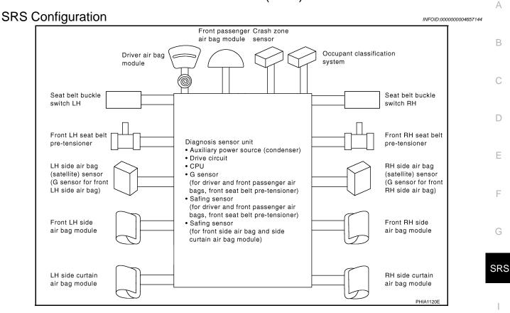
The air bag deploys if the diagnosis sensor unit activates while the ignition switch is in the ON or START position.
