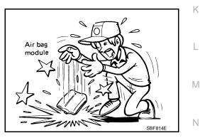
• Always place the side curtain air bag module with the warning label facing upward.
