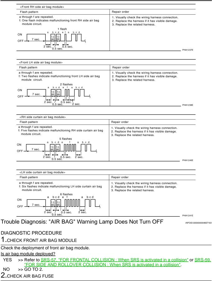
Check 10A fuse [No.13, located in fuse block (J/B)]. Refer to <u>PG-15, "Fuse"</u>.
