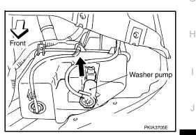
INSTALLATION Installation is the reverse order of removal. CAUTION: When installing washer pump, there should be no packing twists, etc.
