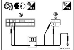
4. Check continuity between IPDM E/R harness connector (A) and Ground.
