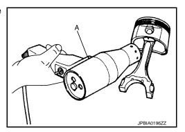
c. Push out piston pin using a stick than has an outer diameter of approximately 20 mm (0.79 in).
