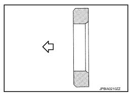
Press-fit pilot bushing (1) as the dimension shown in the figure. (M/T models)
