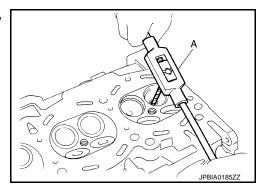
2. If valve seat (EXH) is removed in step 10 (DISASSEMBLY), install it. Replace with oversize [0.5 mm (0.020 in)] valve seat (EXH).
