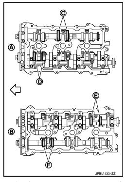
Rotate crankshaft 240 degrees clockwise (when viewed from engine front) to align No. 3 cylinder at TDC its compression stroke.
