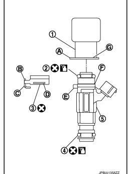
5. Install fuel tube and fuel injector assembly to intake manifold. CAUTION:
