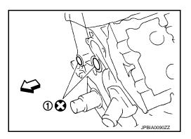
b. Apply liquid gasket with the tube presser (commercial service tool) to rear timing chain case back side as shown in the figure.
