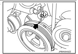
• Check that exhaust cam nose on No. 1 cylinder (engine front side of bank 1) is located as shown in the figure.
