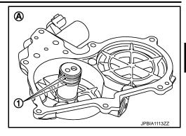
Install intake valve timing control cover with new gasket to front timing chain case.
