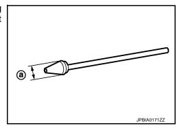
8. With accelerator pedal fully depressed, turn ignition switch to "START" for cranking. When the gauge pointer stabilizes, read the compression pressure and the engine rpm. Perform these steps to check each cylinder.
