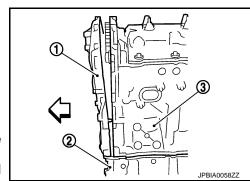
a. Install new seal rings (1) in shaft grooves.
