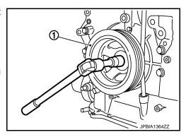
Place suitable puller tab on holes of crankshaft pulley, and pull crankshaft pulley through.
