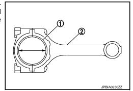
Measure the inner diameter of connecting rod bearing with an inside micrometer.
