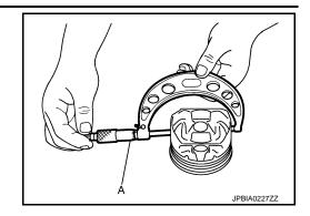
Piston-to-Cylinder Bore Clearance
