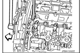
e. Pull stopper pins (C) out from timing chain tensioners (secondary) (1), (2).
