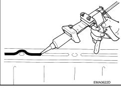
As for bolt holes (B), normally apply liquid gasket inside the holes. Occasionally, it should be applied outside the holes. Check to read the text of this manual.
