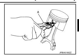
b. Heat piston to 60 to 70°C (140 to 158°F) with an industrial use dryer (A) or equivalent.
