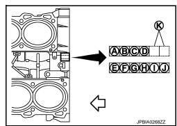
"MAIN BEARING SELECTION TABLE" columns correspond to journal diameter grade on front side of crankshaft.
