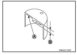
Available thickness of valve lifter (EXH): 27 sizes with range 7.88 to 8.40 mm (0.3102 to 0.3307 in) in steps of 0.02 mm (0.0008 in) (when manufactured at factory). Refer to <a href="EM-145">EM-145</a>, "Camshaft".
