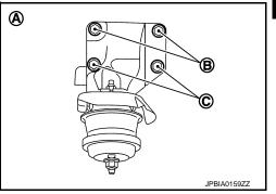
Check that all engine mounting insulators are seated properly, and then tighten mounting nuts.
