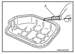
b. Apply a continuous bead of liquid gasket with the tube presser (commercial service tool) to the oil pan (lower) as shown in the figure.
