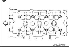
Check the tightening angle using the angle wrench [SST: KV10112100 (BT8653-A)] (A). Never make judgment by visual inspection.
