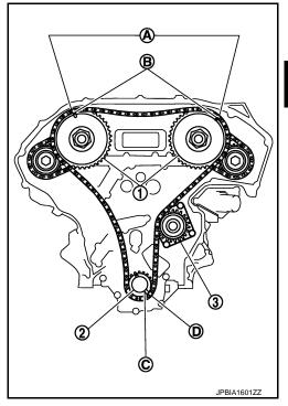
4. Install internal chain guide (1), slack guide (2), and tension guide (3).
