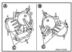
Shaft is engaged with camshaft sprocket (INT) center hole on inside. Pull straight out so that it does not tilt
