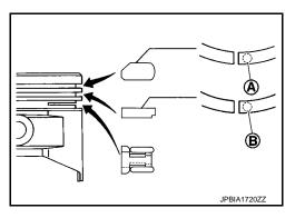
Position each ring with the gap as shown in the figure referring to the piston front mark (D).
