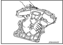
38. Remove old liquid gasket from bolt hole and thread.
