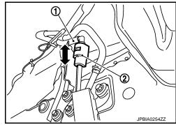
Disconnect guick connector from centralized under-floor piping as follows:
