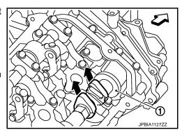
27. Remove crankshaft pulley as follows:
