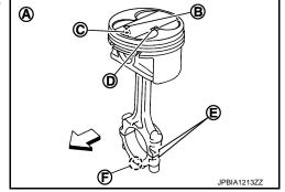
Install new snap ring to the groove of the piston front side.
