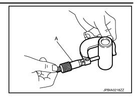
Piston to Piston Pin Oil Clearance
