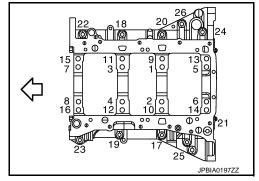
9. Remove lower cylinder block as follows:
