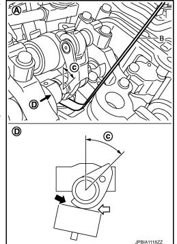
Set No. 1 cylinder at TDC of its compression stroke.
