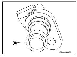
23. Remove intake valve timing control covers and gasket as follows:
