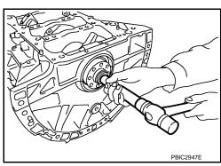
Press-fit pilot converter with its chamfer facing crankshaft as shown in the figure. (A/T models)
