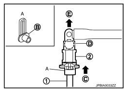
iii. Draw and pull out quick connector straight from centralized under-floor piping.
