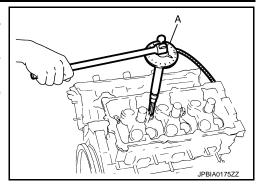
After installing cylinder head, measure distance between front end faces of cylinder block and cylinder head (bank 1 and bank 2).
