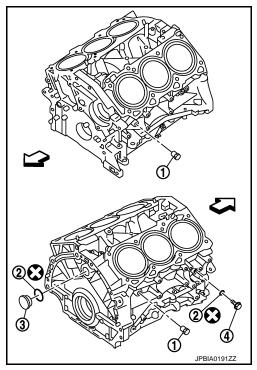
Tighten each plug as specified below.
