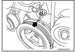
b. Check that exhaust cam noses on No.1 cylinder (engine front side of bank 1) is located as shown in the figure.
