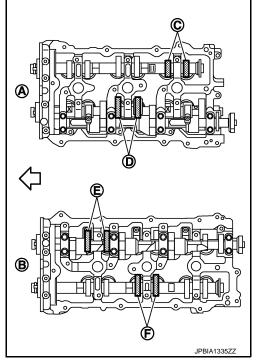
Rotate crankshaft 240 degrees clockwise (when viewed from engine front) to align No. 5 cylinder at TDC of compression stroke.
