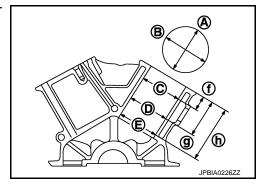
(Clearance) = (Cylinder bore inner diameter) – (Piston skirt diameter).
