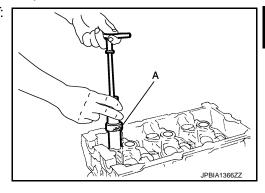
10. Remove valve seat (EXH), if valve seat (EXH) must be replaced.
