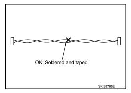
Bypass connection is never allowed at the repaired area.
