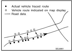
Map-matching does not function correctly when road on which the vehicle is driving is new, etc. and not recorded in the map data. Also, map-matching does not function correctly when road pattern stored in the map data and the actual road pattern are different due to repair, etc.
