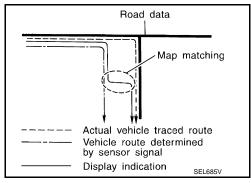
There is a possibility that the vehicle position may not be corrected in the following case, and when vehicle is driven over a certain distance or time in which GPS information is hard to receive. Correct manually the current location mark on the screen.
