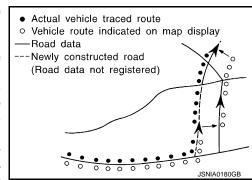
when there is an excessive gap between current vehicle position and the position on the map.
