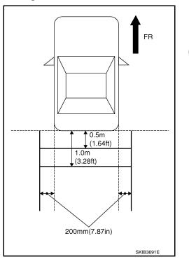
Rotate the center dial, and then select the guiding line pattern so that its angle is aligned with the correction line of the rear of the vehicle.
