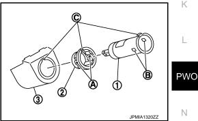
INSTALLATION Install in the reverse order of removal. **NOTE:** Align the cut outs of inner socket, ring, and power socket finisher. **CONSOLE POWER SOCKET**
