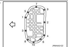
2. Install oil pan drain plug.
