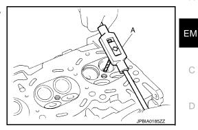
b. Heat cylinder head to 110 to 130°C (230 to 266°F) by soaking in heated oil (A).
