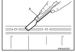
Attach liquid gasket tube to the tube presser (commercial service tool).
