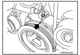
• Check that exhaust cam nose on No. 1 cylinder (engine front side of bank 1) is located as shown in the figure.
