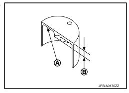
Available thickness of valve lifter (EXH): 27 sizes with range 7.88 to 8.40 mm (0.3102 to 0.3307 in) in steps of 0.02 mm (0.0008 in) (when manufactured at factory). Refer to <a href="EM-144">EM-144</a>, "Camshaft".
