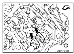
• By referring to the figure, measure the valve clearances at locations marked "x" as shown in the table below (locations indicated in the figure).
