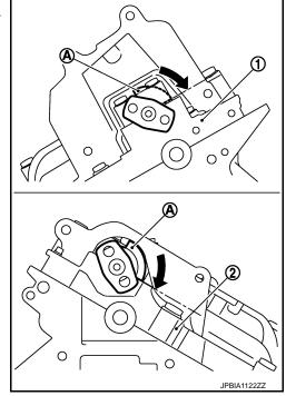
If control shaft cannot be moved, set crankshaft in position referring to the information below. (To displace cam nose)
