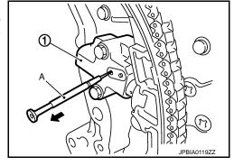
6. Check again that the matching marks on sprockets and timing chain have not slipped out of alignment.
