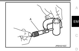
Connecting Rod Bushing Oil Clearance
