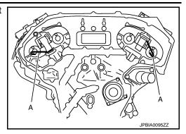
Install timing chains (secondary) and camshaft sprockets.
