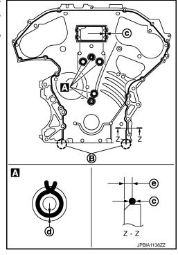
Apply liquid gasket to top surface of oil pan (upper) as shown in the figure.
