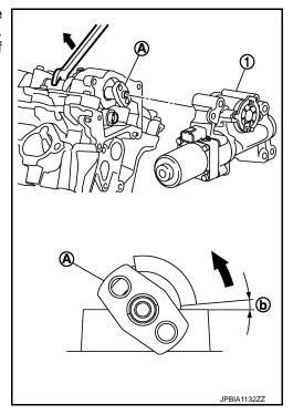
c. Apply a continuous bead of liquid gasket with tube presser (commercial service tool) to the VVEL actuator sub assembly as shown in the figure.
