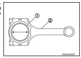
Measure the inner diameter of connecting rod bearing with an inside micrometer.
