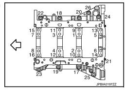
9. Remove lower cylinder block as follows:
