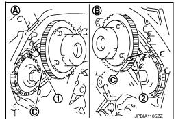
b. Remove camshaft sprocket (EXH) mounting bolt.
