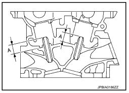
d. Using the valve guide reamer (commercial service tool) (A), apply reamer finish to valve guide (EXH).
