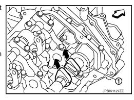
27. Remove crankshaft pulley as follows:
