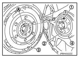
There is a matching mark (B) on the clutch cover side of flywheel (4). Refer it during installation.
