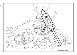
2. If valve seat (EXH) is removed in step 10 (DISASSEMBLY), install it. Replace with oversize [0.5 mm (0.020 in)] valve seat (EXH).
