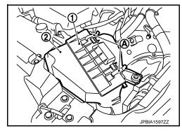
2. Remove holder (3) from air cleaner case (2), and then remove air cleaner filter (1) from holder.
