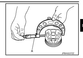
Piston-to-Cylinder Bore Clearance
