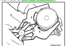
Remove piston from connecting rod as follows:
