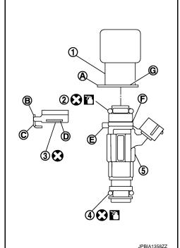
5. Install fuel tube and fuel injector assembly to intake manifold.
