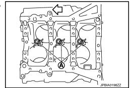
4. Install main bearings and thrust bearings as follows:
