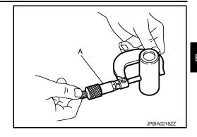
Piston to Piston Pin Oil Clearance
