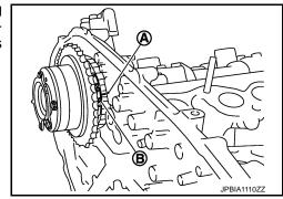
c. Tighten camshaft sprocket (EXH) mounting bolt.
