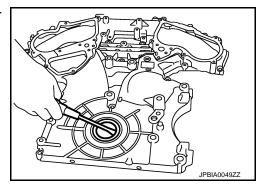
32. Remove O-ring (1) from rear timing chain case.
