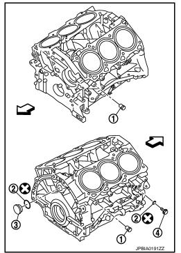
Tighten each plug as specified below.
