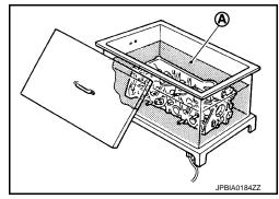
c. Provide valve seats (EXH) cooled well with dry ice. Force fit valve seat (EXH) into cylinder head.
