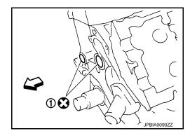
Apply liquid gasket with the tube presser (commercial service tool) to rear timing chain case back side as shown in the figure.
