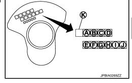
Read the symbol at the cross point of selected row and column in the "CONNECTING ROD BEARING SELECTION TABLE".
