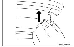
5. Set the tire onto the turntable so that the tire changer arm (2) is at a position approximately 270° from the tire pressure sensor (1).
