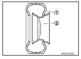
4. Hold tire pressure sensor as shown in the figure, and press the sensor in the direction shown by arrow (←) to bring it into absolute contact with valve hole. After this, tighten valve nut to the specified torque.
