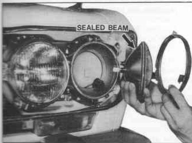
Fig. BE-7 Removing sealed beam
