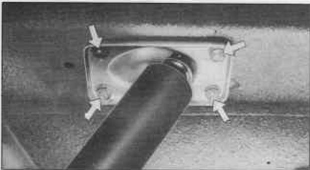
*Fig. RA-41 Removing shock absorber upper bracket*
