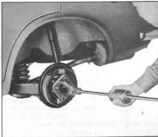
*Fig. RA-16 Removal of rear axle shaft*
