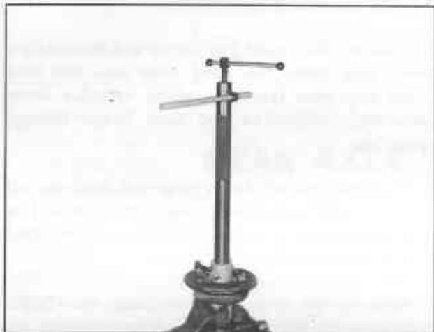
*Fig. RA-30 Removing wheel bearing*
