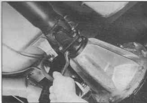
*Fig. RA-26 Removal of companion flange bolts*
