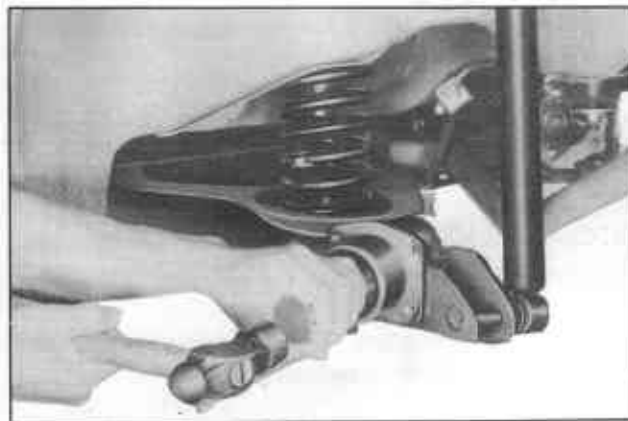
Fig. RA-17 Removing inner bearing using special tool ST49180000
