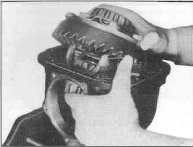
Fig. PD-10 Removing differential case assembly
