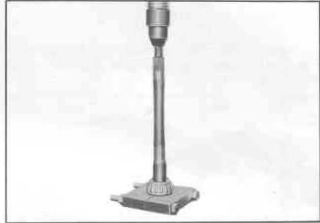
Fig. PD-12 Removing rear bearing inner race
