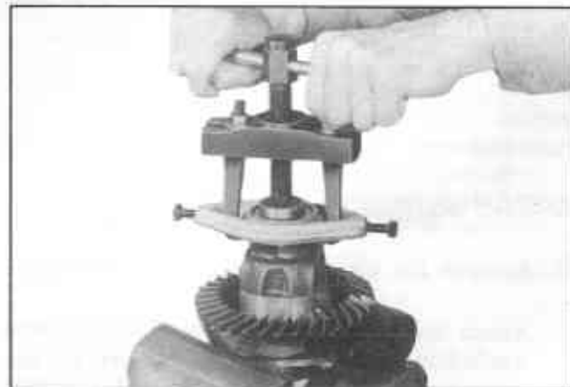
Fig. PD-13 Removing side bearing cone
