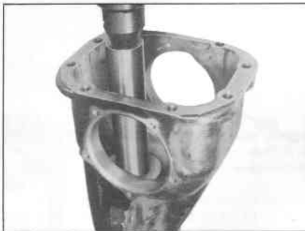
Fig. PD-18 Rear bearing outer race installation
