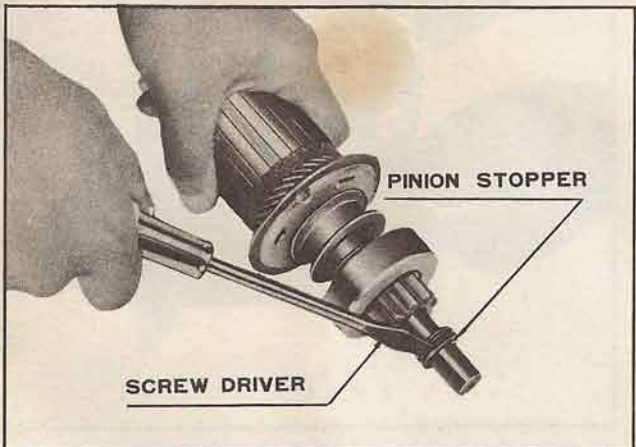
Fig. e Removing Pinion Stopper
