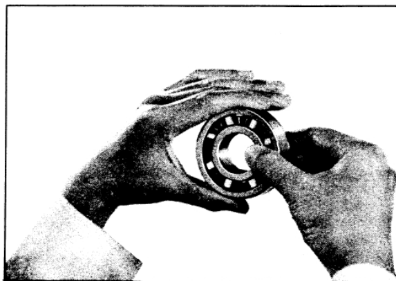
Fig. TM-22 Inspecting ball bearing
