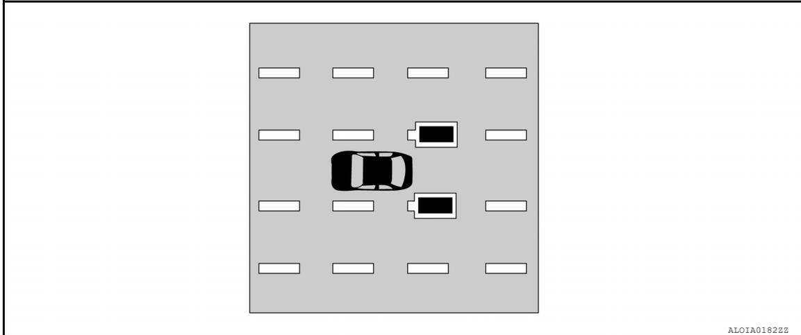
When the vehicle approaches the right lane marker, the driver is alerted by the buzzer and the blinking of lane departure warning lamp (orange).
