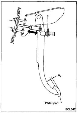
2. Adjust pedal free play with master cylinder push rod. Then tighten lock nut.
