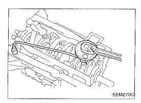
b. Install connecting rod bearing caps.
