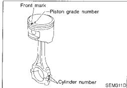
2. Heat piston to 60 to 70°C (140 to 158°F) and assemble piston, piston pin, connecting rod and new snap ring.
