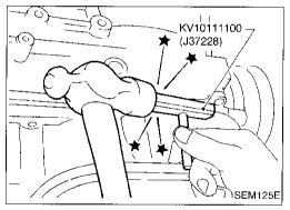
b. Slide Tool by tapping on the side of the Tool with a hammer.
