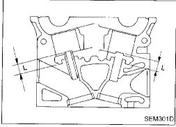
4. Heat cylinder head to 120 to 140°C (230 to 266°F) and press service valve guide onto cylinder head. **Projection** "L":
