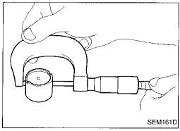
2. Check diameter of valve lifter and valve lifter guide bore. **Valve lifter diameter:**
