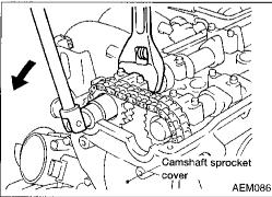
The stoppers on camshaft sprocket cover prevent upper timing chain from disengaging idler sprocket.
