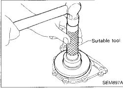
Install new oil seal in the direction shown.
