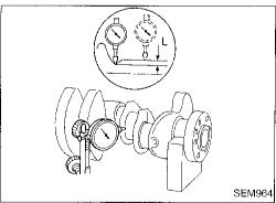
When grinding crankshaft journal, confirm that "L" dimension in fillet roll is more than the specified limit.
