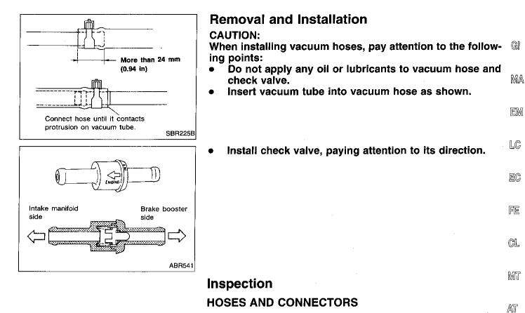
Check vacuum lines, connections and check valve for airtightness, improper attachment, chafing or deterioration.
