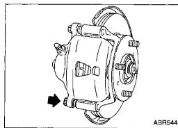
Open cylinder body upward. Then remove pad retainers and inner and outer shims.
