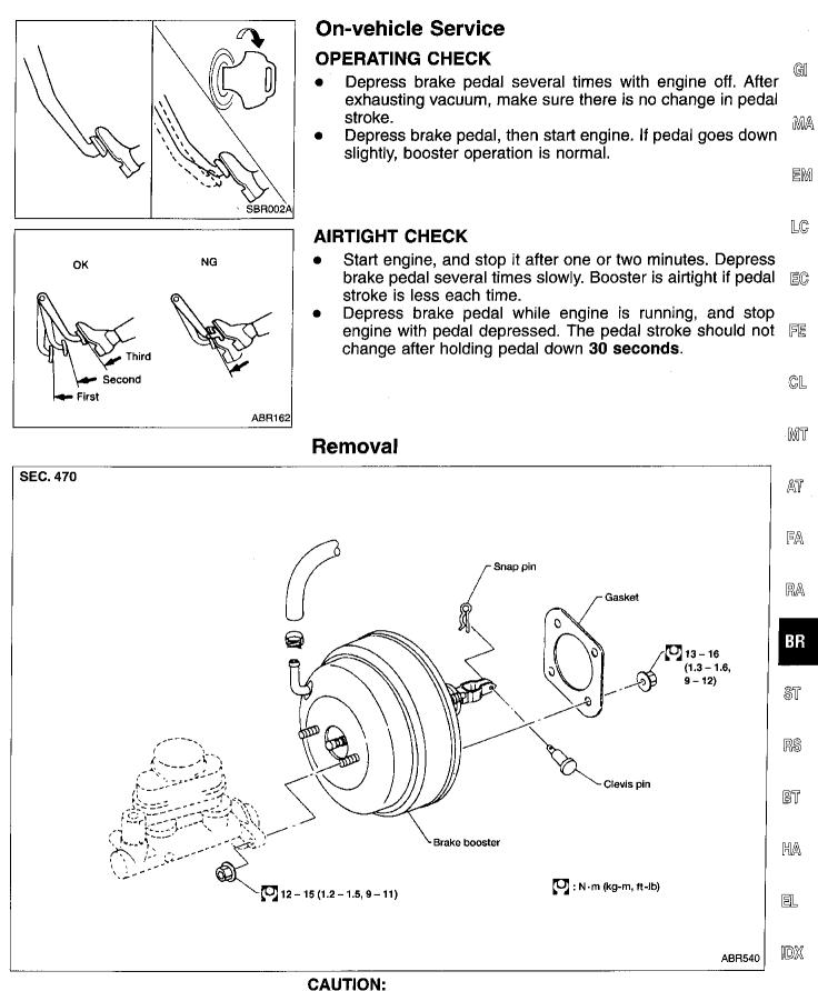
Be careful not to splash brake fluid on painted areas; it may cause paint damage. If brake fluid is splashed on painted areas, wash it away with water immediately.
