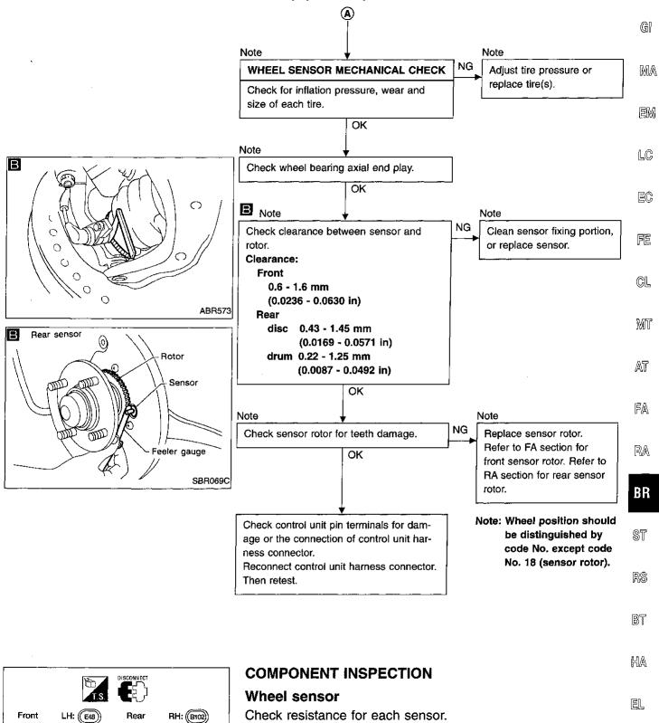
Check resistance for each sensor. Resistance: 0.6 - 3.25 k $\Omega$
