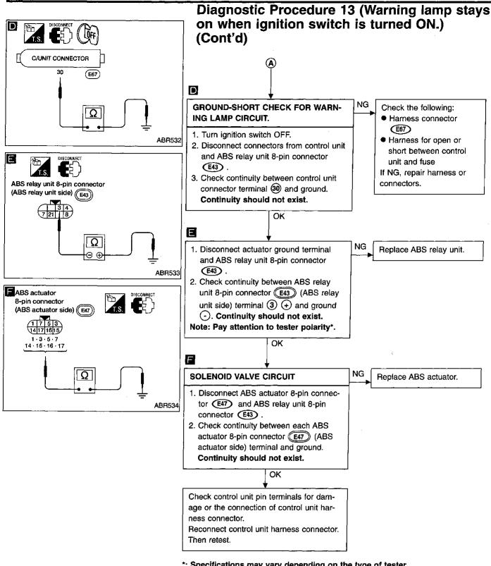
\*: Specifications may vary depending on the type of tester. Before performing this inspection, refer to the instruction manual of the tester.
