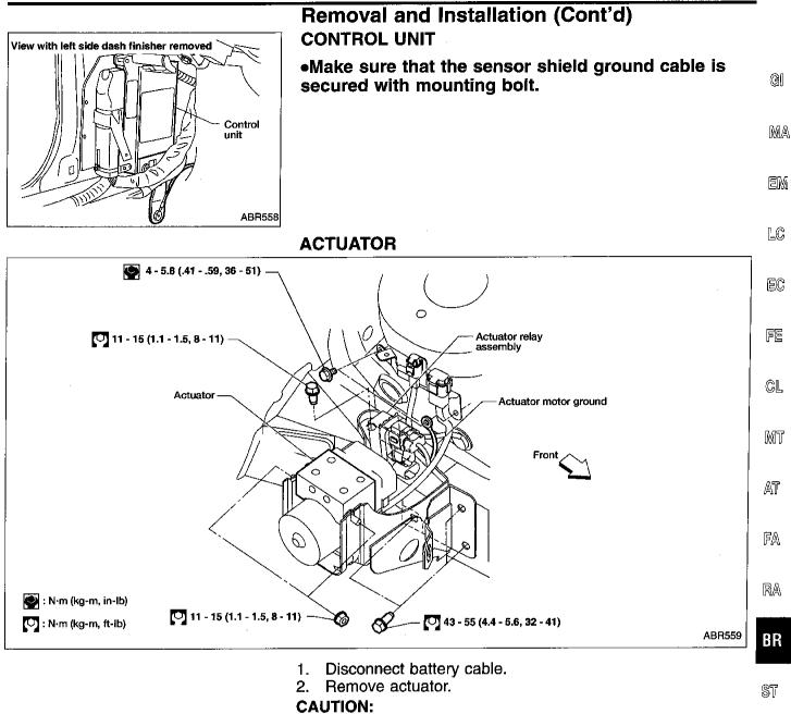
After installation, refill brake fluid and bleed air. Refer to BR-5 and BR-6, respectively.
