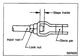
If necessary, adjust brake pedal free height.
