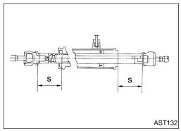
4. Before installing boot, coat the contact surfaces between boot and tie-rod with grease.
