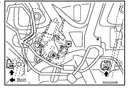
5. While holding the door window, raise it at the rear end to pull the glass out of the sash toward the outside of the door.
