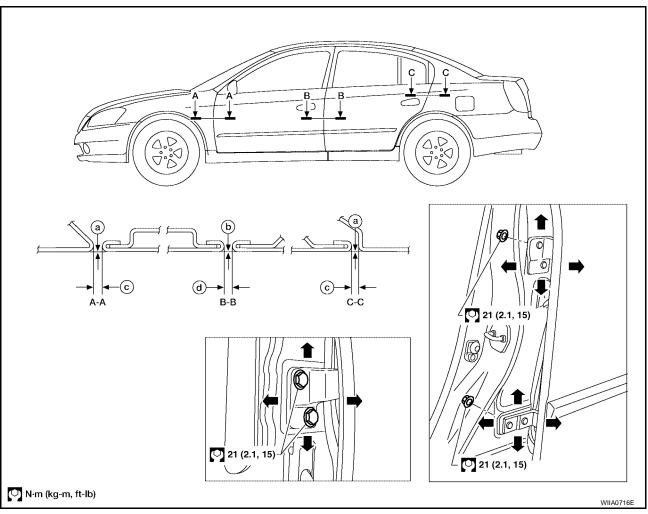
a. Flush + 0.5, -1.0 mm (+0.02, -0.04 in) b. Flush + 1.0, -0.5 mm (+0.04, -0.02 in) c.  $4.5 \pm 1.0$  mm (0.18  $\pm 0.04$  in)
