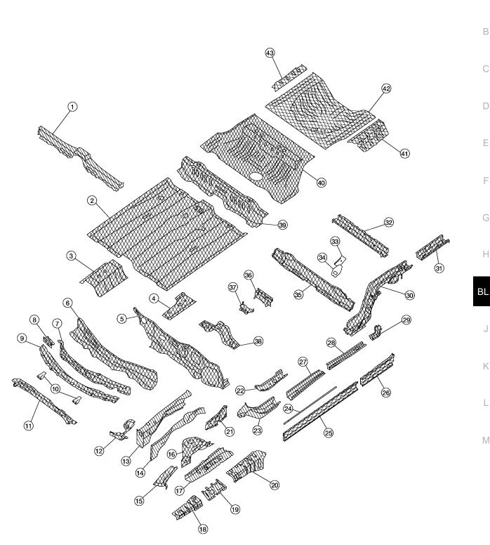
: Indicates both-side anti-corrosive precoated steel portions
