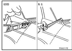
When welding HSS panels, use spot welding whenever possi-GOOD ble in order to minimize weakening surrounding areas due to heat.
