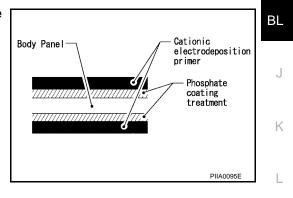
Nissan Genuine Service Parts are also treated in the same manner. Therefore, it is recommended that GENU-INE NISSAN PARTS or equivalent be used for panel replacement to maintain anti-corrosive performance built into the vehicle at the factory.
