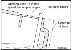
3. Install a new O-ring on the speedometer pinion gear, and install the speedometer pinion gear in to the transaxle case.
