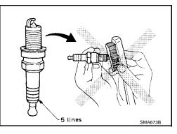
• If the spark plug electrode is covered with carbon, a spark plug cleaner may be used.
