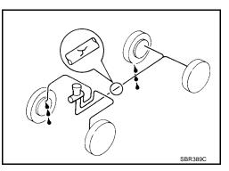
Checking Brake Lines and Cables
