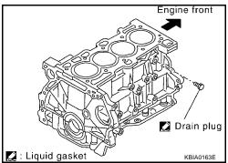
Check the drained coolant for contaminants such as rust, corrosion or discoloration. If the coolant is contaminated, flush the engine cooling system. Refer to <u>MA-17, "FLUSHING COOLING</u> <u>SYSTEM"</u>.
