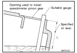
Set a new O-ring on the speedometer pinion gear, then install it in the transaxle case.
