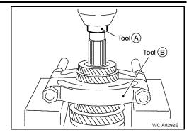
Remove 3rd main gear, 2nd main gear, 2nd needle bearing, 2nd bushing, 1st-2nd synchronizer hub assembly, 1st main gear, reverse main gear, 1st needle bearing, and 1st bushing simultaneously.
