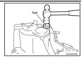
32. Install the new welch plug using Tool as shown.
