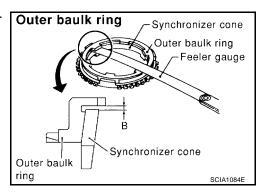
Press the baulk ring on to the clutch gear taper cone by hand, then measure the clearance "C" at two or more points diagonally opposite with a feeler gauge, and then calculate the mean value.
