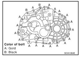
h. Apply gear oil to the O-ring and install it to the control assembly. Then install control assembly to transaxle case. Tighten bolts to the specified torque. Refer to <a href="MT-87">MT-87</a>, "SHIFT CONTROL COMPONENTS"</a>.
