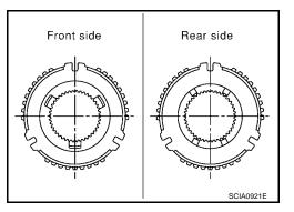
Install with the orientation of the coupling sleeve as shown.
