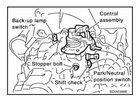
3. After removing shift check and stopper bolt, remove control assembly.
