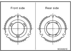
• Do not to hook the ends of the 2 spread springs (front and back have two each) on the same shifting insert.
