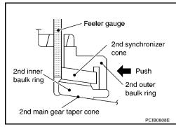
Measure clearance "B" at two points or more on the opposite side using a feeler gauge, then calculate the average.
