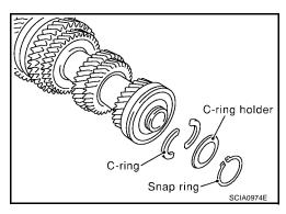
4. Remove the mainshaft rear bearing, adjust shim, and 6th main gear using Tool as shown.
