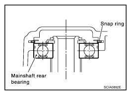
e. Through bore plug mounting hole, with snap ring stretched, lift up mainshaft assembly from the control assembly mounting hole.
