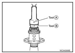
10. Install differential gear into differential case, and tighten final gear bolts.
