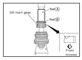
14. Install snap ring onto mainshaft, and check that end play of 5th main gear satisfies standard value.
