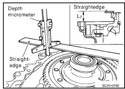
Install the selected adjusting shim and then the differential side bearing outer race using Tool as shown.
