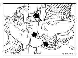
13. Install stopper ring onto 3rd-4th shift fork.
