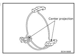
5. Install 1st gear synchronizer assembly onto mainshaft, and synchronizer hub assembly onto mainshaft.
