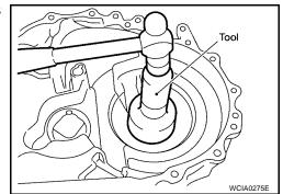
7. Install the final drive assembly into the clutch housing.
