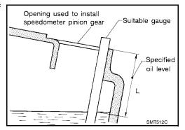
Set a new O-ring on the speedometer pinion gear, then install it in transaxle case.
