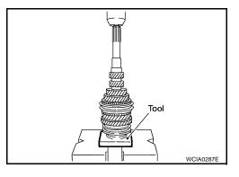
14. Install 5th stopper and then input shaft bearing spacer.
