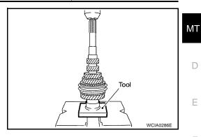
12. Install the synchronizer assembly onto a new 5th-6th synchronizer hub.
