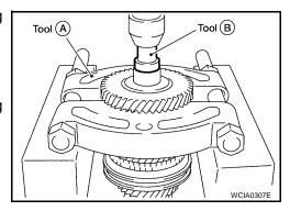
7. Remove the 5th input gear and synchronizer hub assembly simultaneously using Tool as shown.
