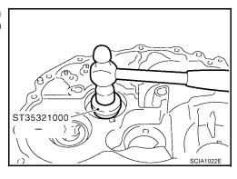
2. Using a drift, install a new differential oil seal.
