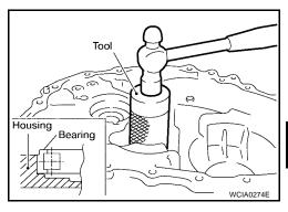
5. Install bearing retainer.
