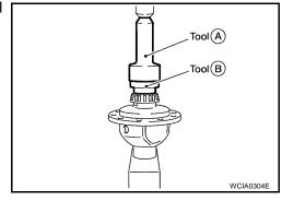
8. Align and install the speedometer drive gear onto the differential case as shown.
