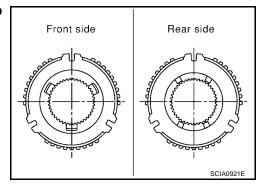
• Install with the orientation of coupling sleeve as shown.
