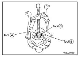
5. Using a pin punch, pull out lock pin and pinion mate shaft as shown.
