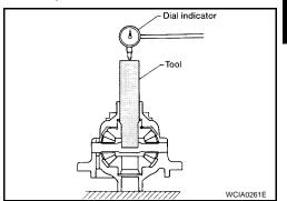
4. Move side gears up and down, and measure the clearance as shown.
