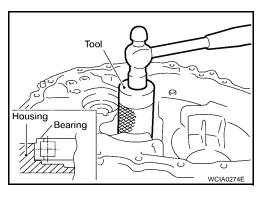
5. Install the mainshaft front bearing retainer.
