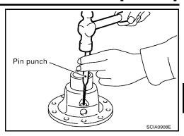
7. Install differential side bearing (transaxle case side) using Tools as shown.
