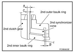
Measure clearance "A" at two points or more on the opposite side using a feeler gauge when pressing baulk ring toward clutch gear taper cone, then calculate the average.
