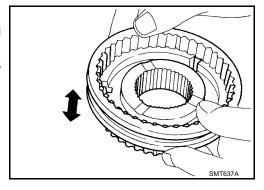
If any crack, damage, or excessive wear is found on the cam face of the baulk ring or working face of the insert as shown, replace it.
