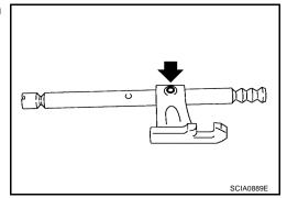
10. Install 1st-2nd fork rod and 1st-2nd shift fork, and then install retaining pin.
