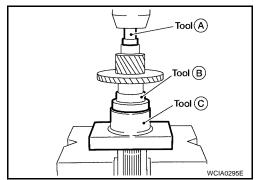
4. Install spread spring, shifting insert and 1st-2nd synchronizer hub onto 1st-2nd coupling sleeve.
