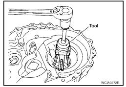
33. Remove input shaft oil seal.
