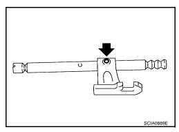
10. Install the 1st-2nd fork rod and the 1st-2nd shift fork, and then install a new retaining pin.
