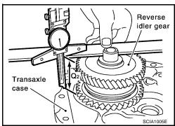
3. Install selected reverse idler gear adjusting shim onto reverse idler gear.
