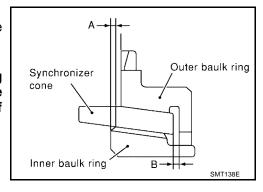
1. Using a dial gauge and Tool, measure clearance "A" at two or more points diagonally opposite, and calculate mean value.
