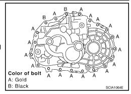
h. Apply gear oil to the O-ring and install it to the control assembly. Then install control assembly to transaxle case. Tighten bolts to the specified torque. Refer to <a href="MT-23">MT-23</a>, "SHIFT CONTROL COMPONENTS"</a>.
