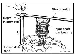
3. Install selected input shaft rear bearing adjusting shim onto input shaft.
