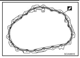
d. With snap ring of mainshaft rear bearing temporarily installed, place transaxle case over clutch housing.
