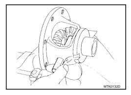
5. Measure end play of side gears using the procedure below, then select a side gear thrust washer.
