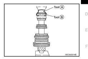
18. Install the C-ring onto the mainshaft, and check that the end play of mainshaft rear bearing meets specifications.
