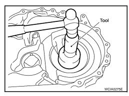
7. Install final drive assembly into clutch housing.
