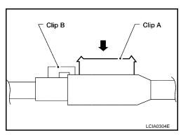
4. Slide clip "B" back over clip "A" until it snaps into place and holds clip "A" in place as shown.
