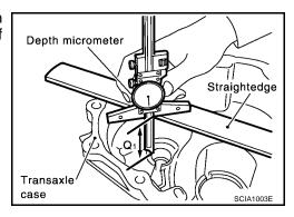
2. Using depth micrometer and straight edge, measure dimension "Q2" between clutch housing case end face and end face of reverse idler gear as shown.
