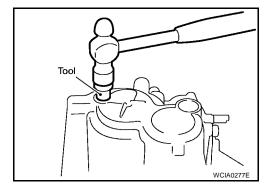
33. Install the 2 check balls, 2 check springs, and the 2 new check ball plugs.
