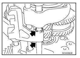
18. Install a new retaining pin onto the 5th-6th shift fork.
