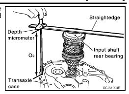
3. Install the selected input shaft rear bearing adjusting shim onto the input shaft.
