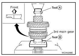
11. Select suitable adjusting shim so that dimension "C1" satisfies standard value below, and install it onto mainshaft.
