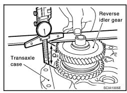
3. Install the selected reverse idler gear adjusting shim onto the reverse idler gear.
