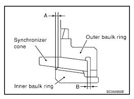
Using a dial gauge, measure clearance "A" at 2 or more points diagonally opposite, and calculate mean value.
