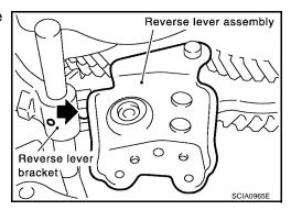
c. Tighten the bracket bolts to specification, and install the reverse lever assembly.
