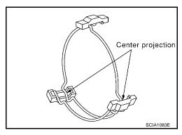
5. Install the 1st gear synchronizer assembly onto the mainshaft, and the synchronizer hub assembly onto the mainshaft using Tool as shown.
