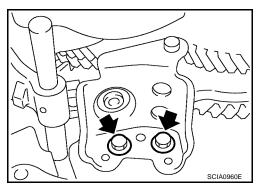
25. Install the check ball, reverse shift check sleeve, reverse check spring, and the reverse check ball plug.
