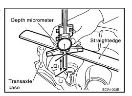
2. Using a depth micrometer and straight edge, measure the dimension "Q2" between the clutch housing case end face and the end face of reverse idler gear as shown.
