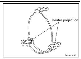
4. Install the 3rd-4th synchronizer assembly using Tool as shown.
