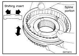
If any cracks, damage, or excessive wear is found on the cam face of baulk ring or working face of the insert as shown, replace it.
