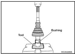
8. Measure the dimension "C2" as shown. Select a suitable thrust washer so that dimension "C2" satisfies the standard dimension specification. Then install the thrust washer onto the input shaft.
