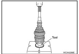
15. Install snap ring onto input shaft, and check that end play (gap between snap ring and groove) of input shaft bearing spacer satisfies standard.
