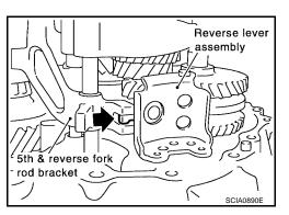
c. Tighten mounting bolts to specified torque, and then install reverse lever assembly.
