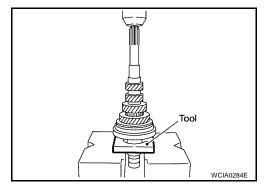
5. Install the 4th bushing using Tool as shown.
