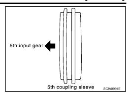
Be sure not to hook ends of 2 spread springs (front and back have two each) on same shifting insert.
