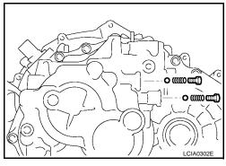
34. Apply sealant to the threads of the park/neutral position switch and back-up lamp switch. Then install them into the transaxle case. Refer to <a href="MT-84">MT-84</a>, "CASE AND HOUSING COMPONENTS"
