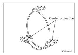
13. Install 5th synchronizer hub assembly.
