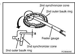
Measure clearance "C" at two points or more on the opposite side using a feeler gauge when pressing baulk ring toward clutch gear taper cone, then calculate the average.
