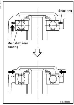
f. Securely install snap ring onto mainshaft rear bearing.
