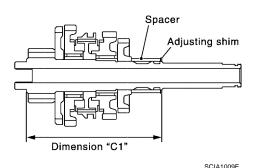
Standard length "C1" 173.85 - 173.95 mm (6.844 - 6.848in) Thickness mm (in) Part number\* Thickness mm (in) Part number\* 0.52 (0.0205) 32238 8H500 0.84 (0.0331) 32238 8H504 0.60 (0.0236) 32238 8H501 0.92 (0.0362) 32238 8H505 0.68 (0.0268) 32238 8H502 1.00 (0.0394) 32238 8H506 0.76 (0.0299) 32238 8H503 1.08 (0.0425) 32238 8H507
