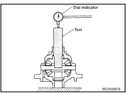
c. Move side gears up and down to measure end play, and select thrust washer so that it meets specification.
