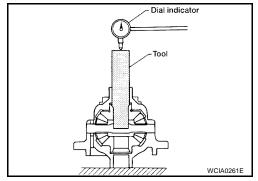
c. Move side gears up and down to measure end play, and select thrust washer so that it satisfies standard.
