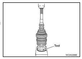
17. Install input shaft front bearing.
