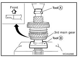
11. Measure the dimension "C1" . Select a suitable adjusting shim so that the dimension "C1" satisfies the standard dimension specification, and install it onto the mainshaft.
