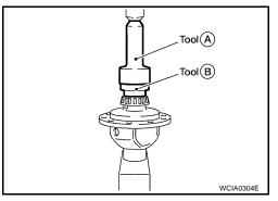
8. Align and install speedometer drive gear onto differential case.
