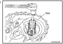
37. Remove the input shaft oil seal using a suitable tool as shown.
