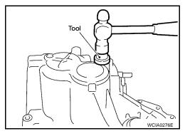
27. Using Tool, install a welch plug as shown.
