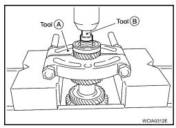
6. Remove the 4th main gear and 5th main gear simultaneously using Tool as shown.
