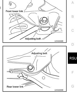
2. Tighten the adjusting bolt nuts to the specified torque.
