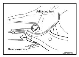
8. Tighten the adjusting bolt nuts to the specified torque.
