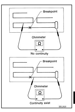
To locate a break, move probe along element. Tester indication 3. will change abruptly when probe passes the broken point.
