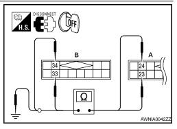
4. Check continuity between satellite radio tuner (factory installed) and ground.
