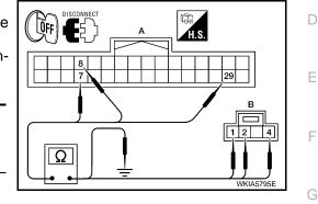
4. Check continuity between Bluetooth control unit harness connector B126 (A) and ground.
