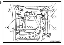
5. Pull out the navigation audio unit assembly, disconnect the navigation audio unit assembly connectors.
