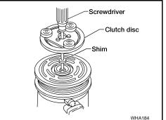
4. Install the clutch disc on the drive shaft, together with the original shim(s). Press the clutch disc down using the drive plate installer.
