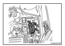
While depressing the tabs (A) remove the IPDM E/R (1) from the vehicle.
