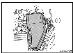
Disconnect the harness connectors from the IPDM E/R.
