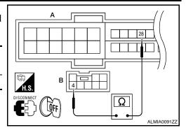
3. Check continuity between IPDM E/R harness connector and ground.
