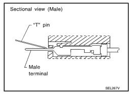
How to Check Enlarged Contact Spring of Terminal
