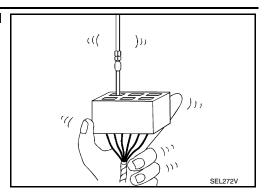
If the male terminal can be easily inserted into the female terminal, replace the female terminal.
