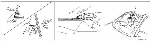
If the windshield glass is to be reused, mark the body and the glass with mating marks.
