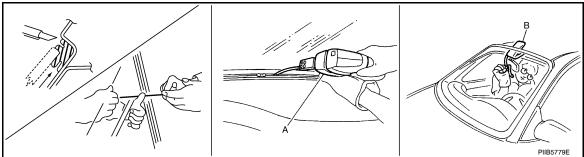
If the rear window glass is to be reused, mark the body and the glass with mating marks.
