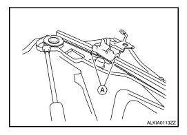
• Apply grease for each sliding part. Apply grease at the application points (A) as shown.
