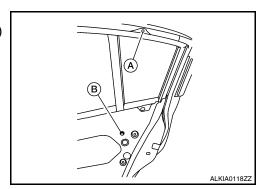
8. Remove the partition glass from the inside of the door in the direction as shown.
