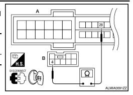
Check continuity between IPDM E/R harness connector and ground.
