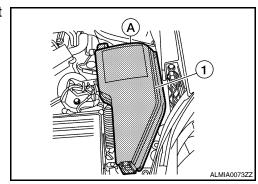
Disconnect the harness connectors from the IPDM E/R.
