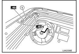
4. Check that the wind deflector (1) moves freely within the sunroof unit assembly while manually pressing down and releasing. If a malfunction is detected, remove the sunroof unit assembly and visually inspect; refer to <u>RF-91</u>, "<u>Inspection</u>". If damage is found, replace either wind deflector (1) or sunroof unit assembly as required.
