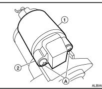
3. Connect the terminal "M" connector and tighten terminal "M" nut (A) to specification.
