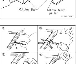
Determine cutting position and record distance from the locating indent. Use this distance when cutting the service part. Cut outer front pillar over 60 mm above inner front pillar cut position.
