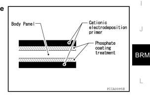
Nissan Genuine Service Parts are also treated in the same manner. Therefore, it is recommended that GENU-INE NISSAN PARTS or equivalent be used for panel replacement to maintain anti-corrosive performance built into the vehicle at the factory.
