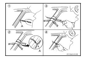
Determine cutting position and record distance from the locating indent. Use this distance when cutting the service part. Cut outer front pillar over 60 mm above inner front pillar cut position.
