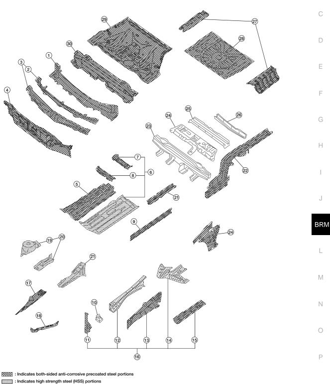
: Indicates both-sided anti-corrosive steel and HSS portions
